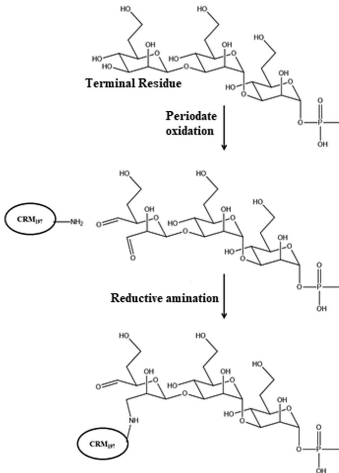
Figure 4. Conjugation of *C. jejuni* HS53 CPS to protein carrier CRM<sub>197</sub> by periodate oxidation/reductive amination method. The monosaccharide at the non-reducing end was first oxidized with periodate and then conjugated coupled to a protein by reductive amination (49).
